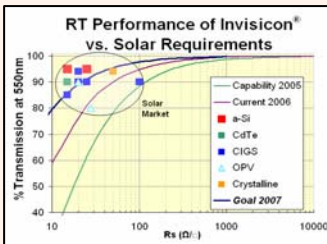
Fig. 3. RT performance of Invisicon ® Transparent Coatings
